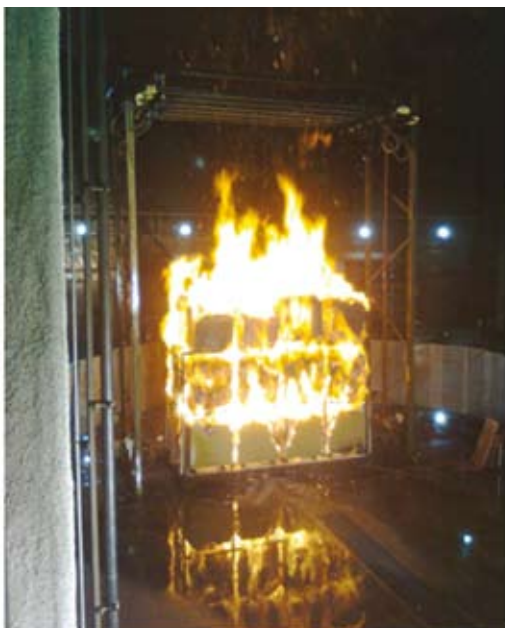
Figure 1: Fire testing at the FM Global Research Centre, fire on storage racks without any form of active fire protection. The fire was well developed within five minutes
